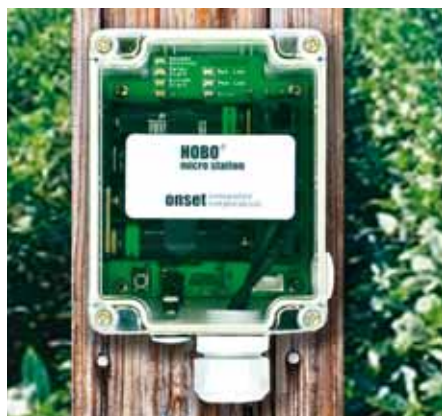
HOBO Micro Station H21-002 8.9 x 11.4 x 5.4 cm (3.5 x 4.5 x 2.125 in) 0.5 kg (1 lb)
