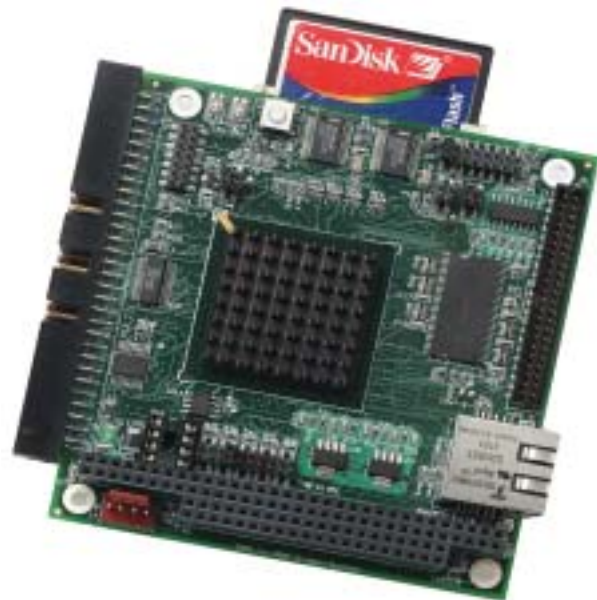
Octagon Systems' highly integrated PC/104 package with CompactFlash™.
